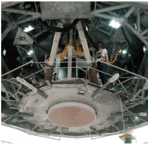
Figure 5 (Color online) The 19-beam 1.05-1.45 GHz receiver installed on the lower platform of the Stewart manipulator.
