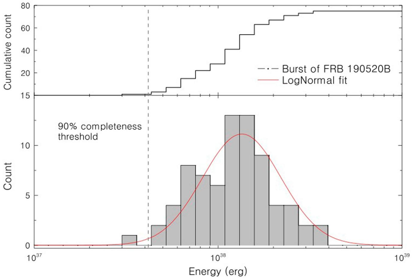
**Extended Data Fig. 6 | The distribution of burst energies for FRB 20190520B.** The bursts are from FAST observations. The red line and black dashed line are the log-normal fit and 90% completeness threshold,
