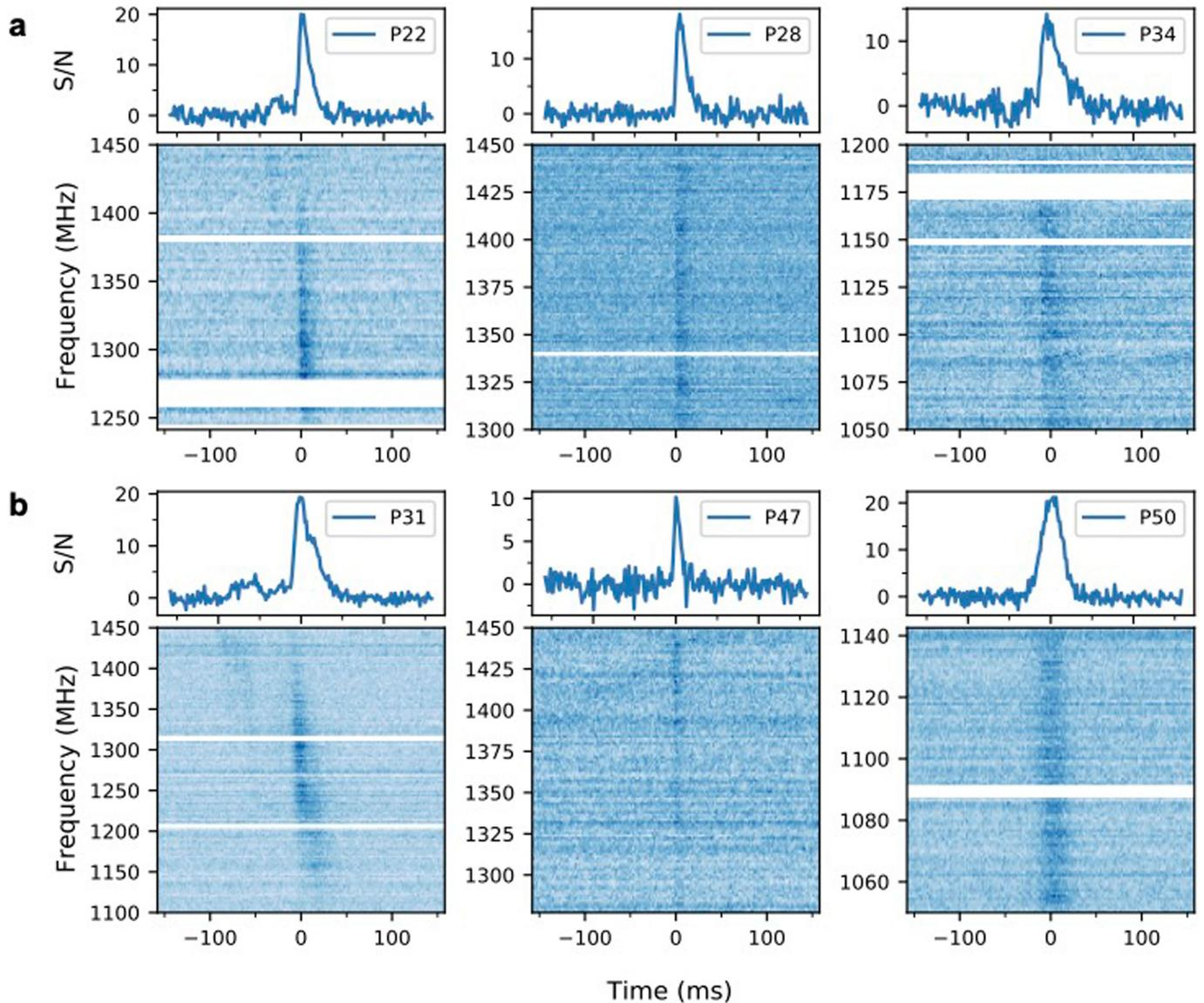
**Extended Data Fig. 7 | Dynamic spectra of bursts with and without scattering. a,** Frequency-time dynamic spectra of bursts with significant evidence of pulse broadening, along with 1D burst profiles that have been averaged across the entire frequency band. **b,** Examples of bursts without significant evidence of pulse broadening. White lines indicate excised radio frequency interference. All 1D burst profiles are shown in units of the
